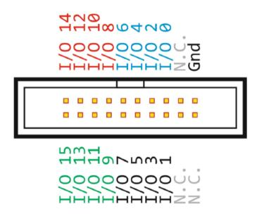
Figure 4 Pin Layout for Logic Connector (Tracker)
