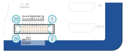
Pinout for IO Probe Connector (Explorer)
