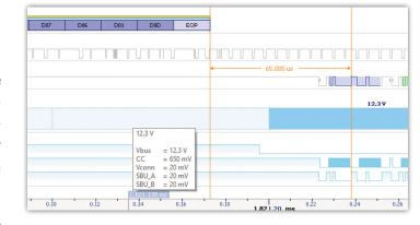
External logic signals can be captured over the Logic/ GPIO connection and displayed in discrete formats and in grouped bus formats, in synchronization with all other events captured. Bus throughput information is also provided to assist with characterizations of data transfer is-
