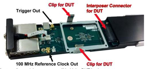
The two clips and the connector will hold the DUT in place.
